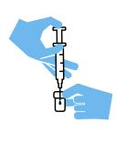
**2. Inject** the sample solution into the cuvette.
